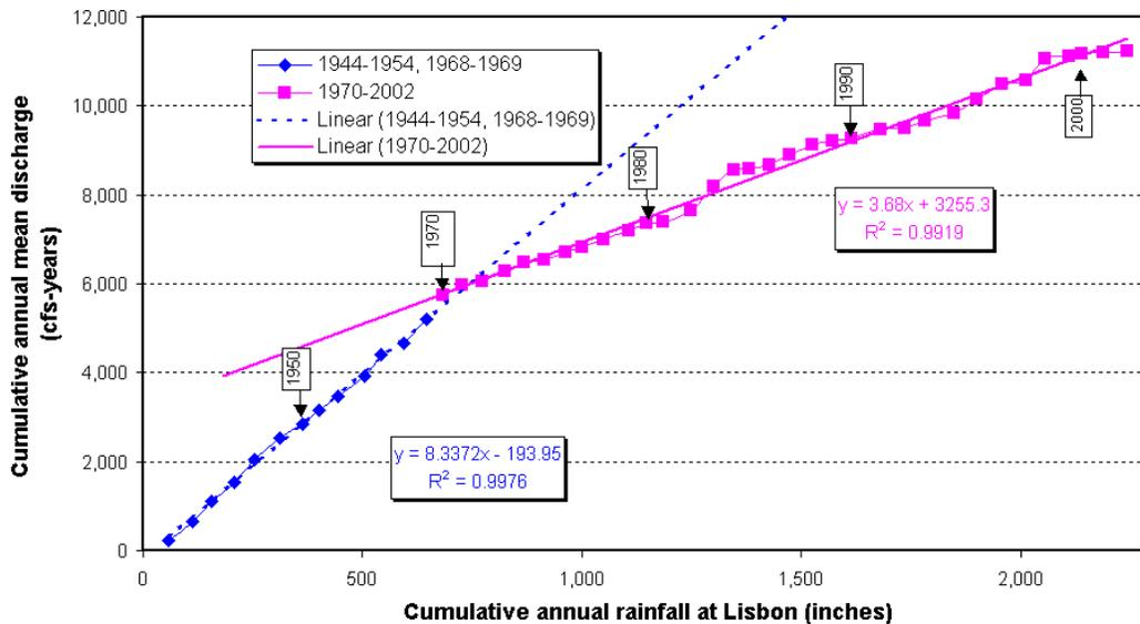
**Figure 6. Double-mass curves for Ocklawaha River discharge at Moss Bluff vs. Lisbon rainfall (Only years with complete discharge records are plotted)**
