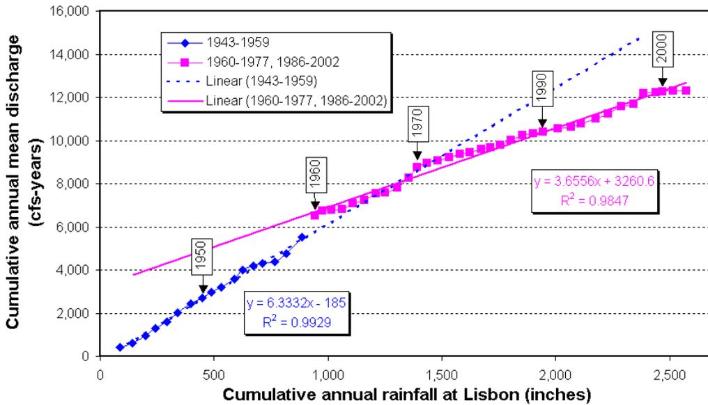
**Figure 7. Double-mass curves for Haines Creek discharge vs. Lisbon rainfall**
