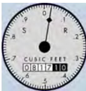
Figure A-1. Simple dial meter in cubic feet.
